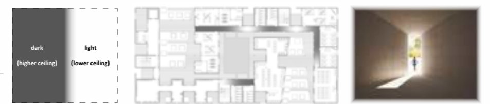
"Ceiling Design: the ceiling of corridor is designed into wavy shape (the lighter the lower, the darker the higher) to emphasize the lighting special atmosphere within corridor. The plan (scale 1:400) showing how the wavy corridor ceiling is designed in the 1st floor. (Reference picture for showing the atmosphere of this ceiling design: the picture from the designing: dl atelier outdoor orchestra stage)"
