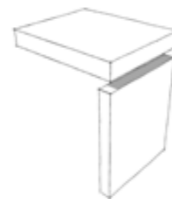
cantilever roof is projected from wall
