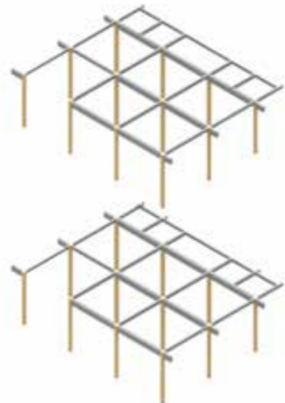
"# Major Structure: Steel Frame Structure with Cantilevered Balcony (for light-weight and large span) # Structure System: Column Grid System # Structural Module: 0.9m"
