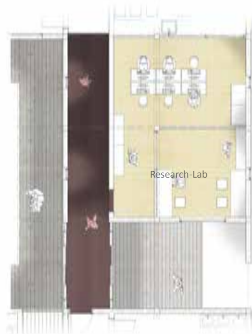
"Detailed Plan: The Area around Research-Lab (1st Floor; Indicating by Dashed Square in the 1st Floor Plan) (Showing the Texture of Floor, Lighting Condition, Beam and Skylight Layout Above) (Scale 1:50)"
