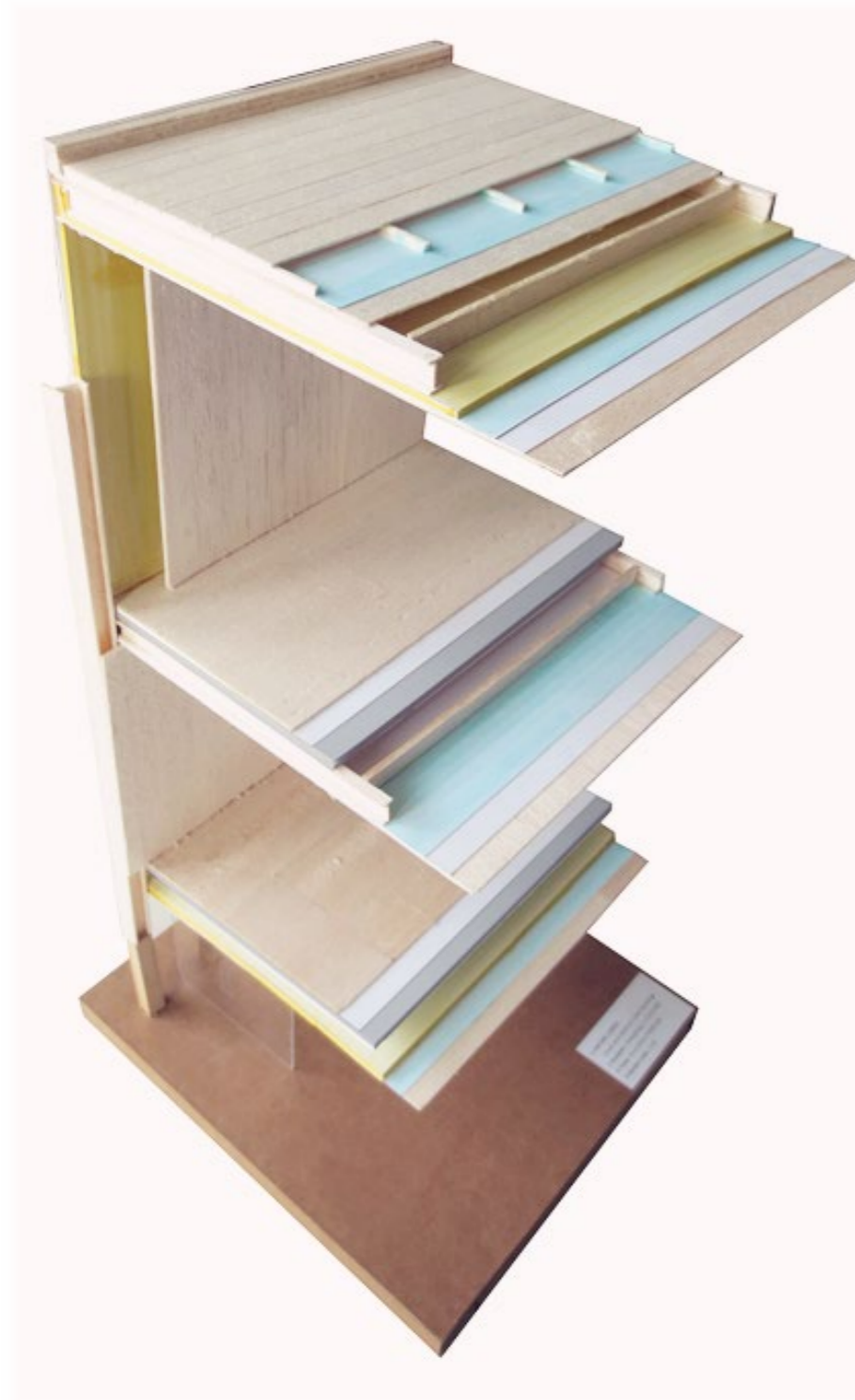
“The 1:20 Tectonic Model Shows The Main Construction Details Of This Project (Including Roof, Floor, Lifted Floor And Wall Constructions)”
