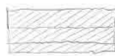
#3 THE TOTAL THICKNESS OF 3 DIFFERENT STONE LAYERS IS CERTAIN FOR ACHIEVING SAME HEIGHT OF FACADE
